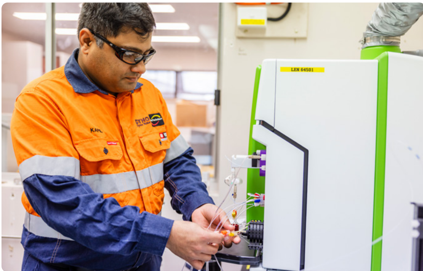
Incitec Pivot Laboratory Quality Coordinator, Kapil Dubal, preparing and adjusting an ICMS instrument to measure micronutrients and heavy metals in fertiliser samples.
