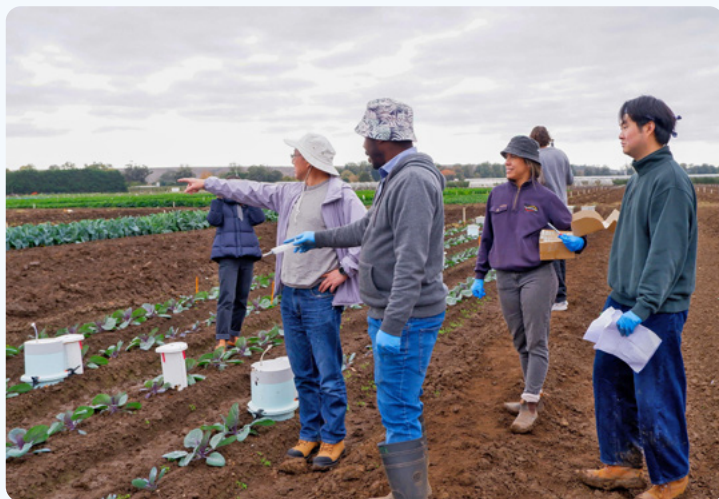
University of Melbourne's Professor Deli Chen, with IPF's Dr Robert Impraim and Natalia Gomez; and University of Melbourne student and IPF intern, Bo-Lung You, inspecting chambers covering cauliflowers, that measure greenhouse gases CO 2 (carbon dioxide), N 2 O (nitrous oxide), CH 4 (methane), and NH 3 (ammonia).
